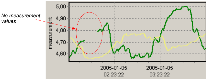
Fig. 3.10. Interruption in the graph (e.g. sensor fault)
