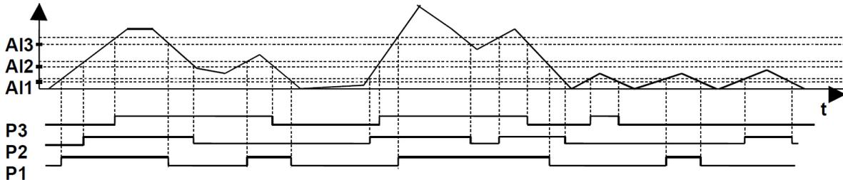
Figure 17. Operation of the algorithm for 3 alarms/relays
