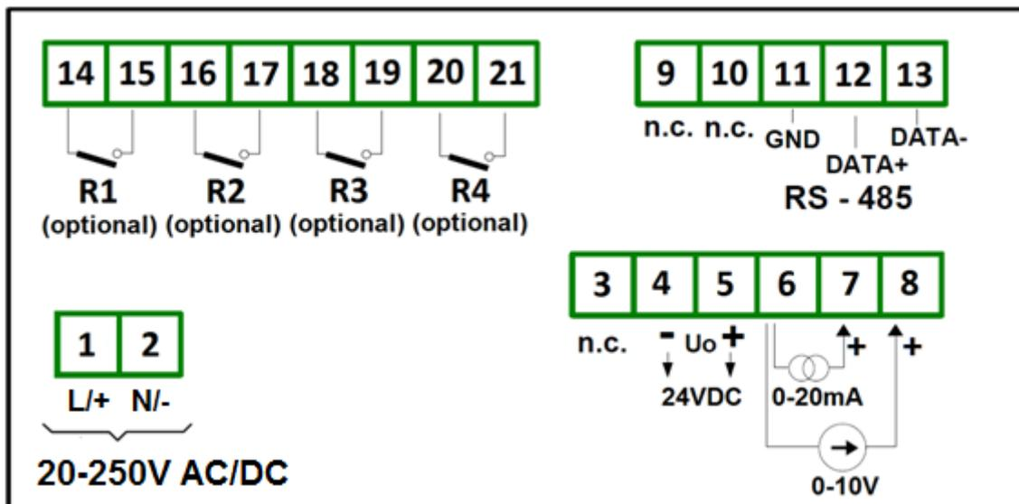
Figure 6. Description of terminals for standard version
