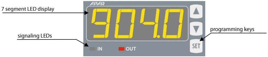
Fig.8. Description of the front elevation
