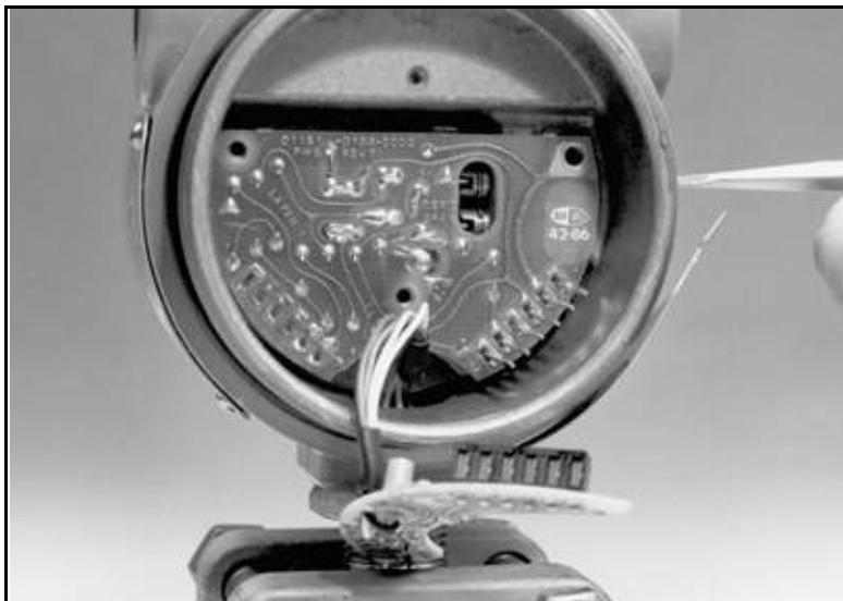
8. For linear output models, grip the calibration board (5) by the interface pin. (Removing the calibration board disables the conventional zero and span screws.)
