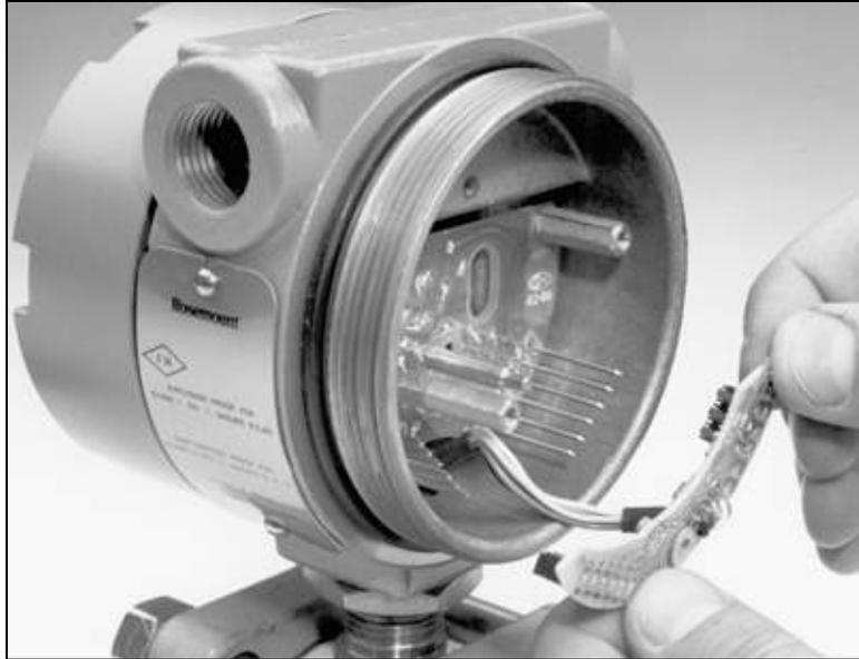
6. If the transmitter has linear output electronics, remove the three standoffs (4). Use a 1/4-in. nut driver or wrench.
