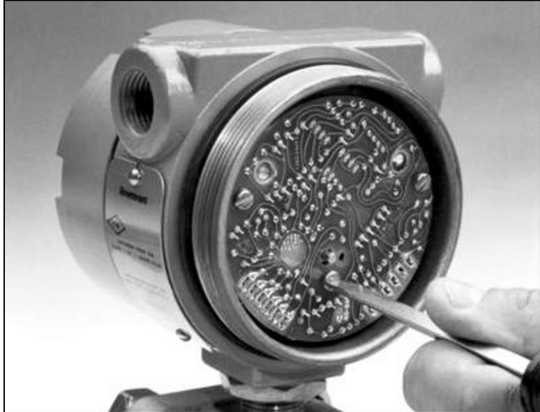
4. Pull the amplifier board (2) or amplifier/squaring assembly (13) directly off the bayonet connectors (6).
