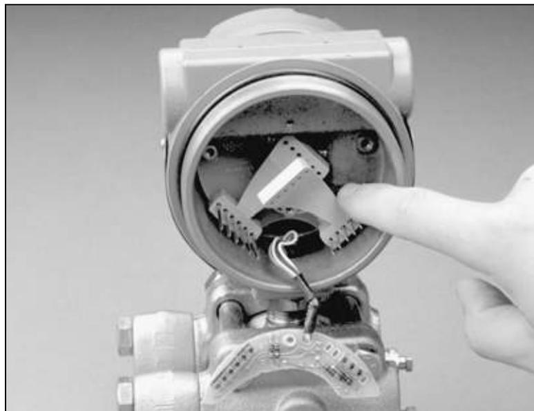
2. Align the header board with the bayonet connector pins, and slide the header board halfway down the pins.
